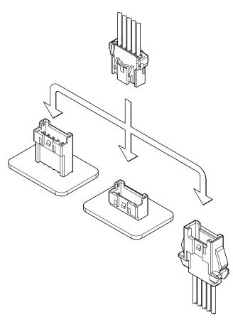
XAF connector is an insulation displacement socket connector which is compatible with the existing XA connector crimp housing (plug housing). The dipping type, SMT type, and high box type headers or the receptacle housings used for wire-to-wire connection can be prepared as the mated counterpart of XAF connector, and the wide range of connection style can be provided depending on the application.
