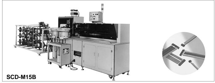
This SCD-M15B series machine can make the hybrid harnesses which consist of shielded wires and discrete wires that effectively reduce the crosstalk or electromagnetic interference inside of the electronic equipment.
