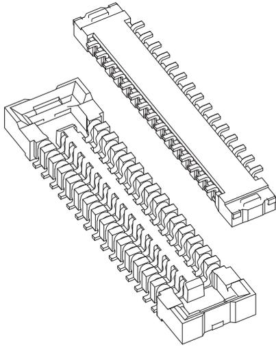
**This is space saving type board-to-board connector with 0.4mm pitch, 0.8mm between PC boards and 2.0mm product width. 1.0mm Between PC boards is available by using dedicated receptacle.**
