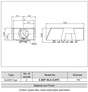
Housing: Thermoplastic resin, UL94-HB, black Lock piin: Stainless
