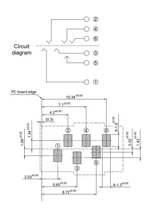
Note:1. The above figure is the figure viewed from the connector mounting side. 2. Tolerances are non-cumulative: ±0.05 mm for all centers. The dimensions above should serve as a guideline. Contact JST for details.
