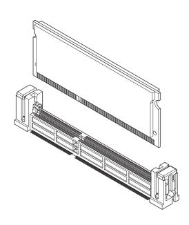
Socket for DDR/DDR3 S.O.DIMM 204circuit complying with JEDEC (MO-268). Hold the PC board by the mechanism for preventing to come off the PC board. Mechanism for preventing incomplete mating to check by visual from upper, and right and left is provided.
